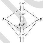
Equivalent capacitance =  $4 \times 6 = 24 \mu F$
