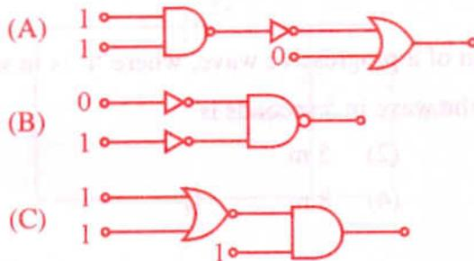
In the following combination of logic gates, the outputs of A, B and C are respectively
