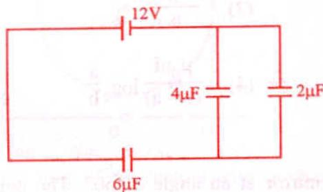
The charge deposited on  $4 \mu\text{F}$  capacitor in the circuit is
