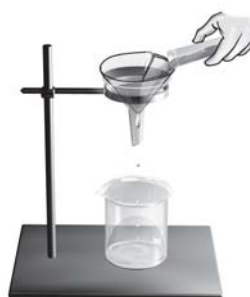
Fig. 5.10 Filtration using a filter paper
