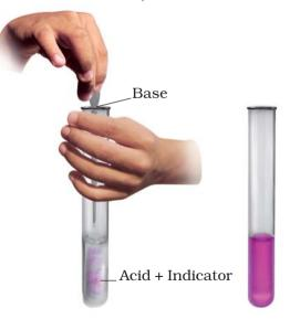
Fig. 5.4 Process of neutralisation
