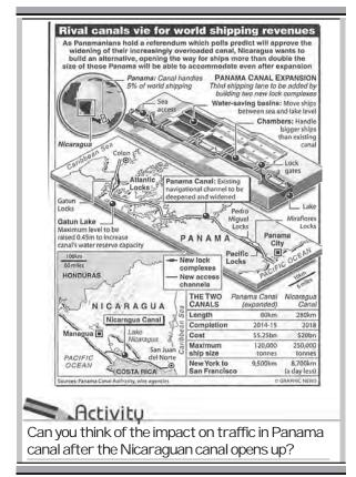
constructed across the Panama Isthmus between Panama City and Colon by the U.S. government which purchased 8 km of area on either side and named it the Canal Zone. The Canal is about 72 km. long and involves a very deep cutting for a length of 12 km. It has a sixlock system and ships cross the different levels (26 m up and down) through these locks before entering the Gulf of Panama.
