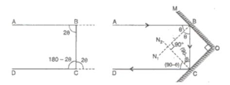
It is clear from the geometry that AB || CD i.e., incident ray AB is parallel to reflected ray CD but the direction is reversed.
