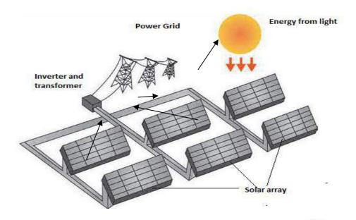
**b.** Energy conversion in photovoltaic cell: Electric energy can be produced directly from sunlight without the application of principle of electromagnetic induction through solar photovoltaic cells. These cells convert solar energy directly into electrical energy through the solar photovoltaic effect. The electrical energy thus produced is DC in nature. The energy has to be stored to be in batteries for later use, since the energy production is dependent on sun light.
