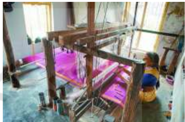
Fig. 8 A Jamdani sari on loom. Weft being woven over warp.
