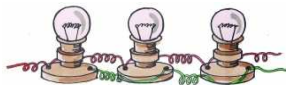
Fig. 13 - bulbs connected in parallel
