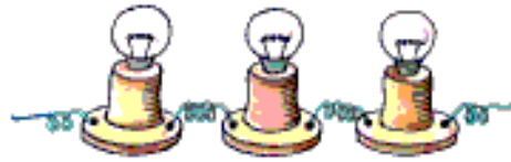
Fig. 12 - Bulbs connected in series
