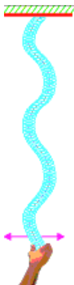
Fig-5 Transvers waves in a slinky
