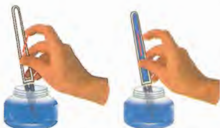
Atmospheric pressure presses liquid into the dropper (filler)
