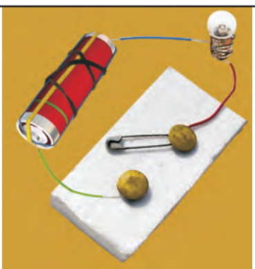
Fig 12.9 An electric circuit with a switch
