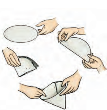
Fig 5.9 Folding filter paper to make a cone
