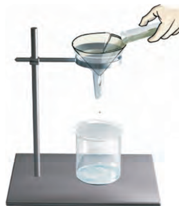
Fig 5.10 Filtration using a filter paper
