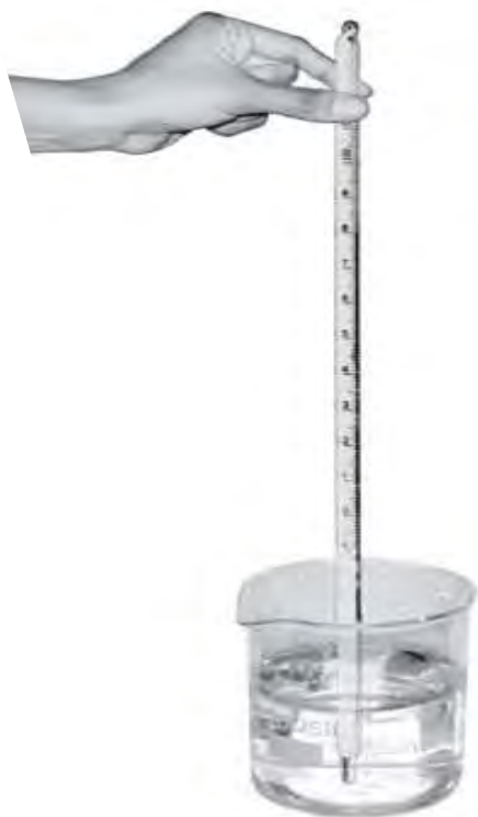
Fig.4.5: Measuring temperature of water with a laboratory thermometer
