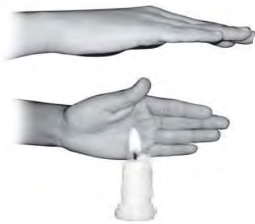
Fig.4.10: Transfer of heat by convection in air
