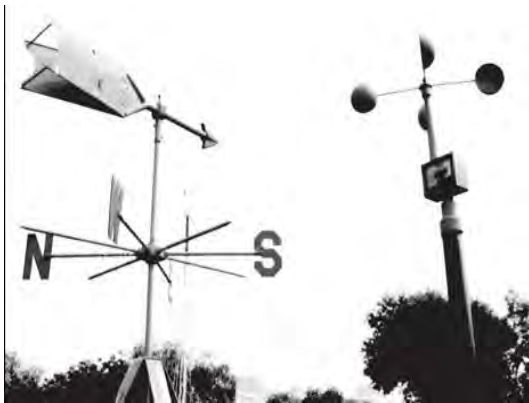
Fig. 8.17 : An anemometer for measuring the speed of wind Courtesy : India Meteorological Department, New Delhi
