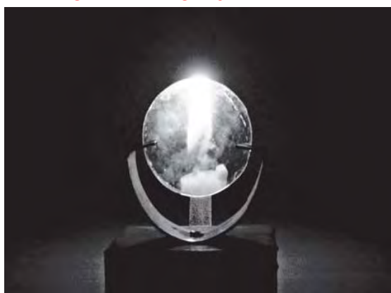
Fig.15.26: A virtual image formed by the convex lens
