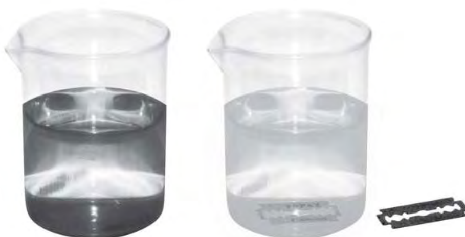
Fig.6.4: Change in colour of the copper sulphate solution due to reaction with iron
