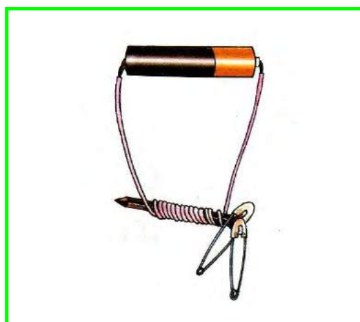
Fig.14.8: An Iron nail attracts more safety pins when wrapped with a coil with more number of turns
