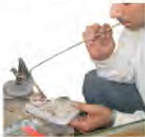
Fig. 6.11 : Goldsmith Blowing Through a Metallic Pipe
