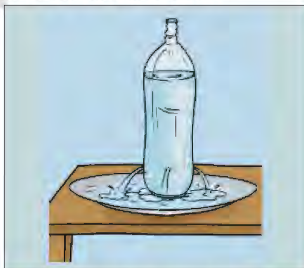
Fig. 9.16 : Liquids Exert Equal Pressure at the Same Depth
