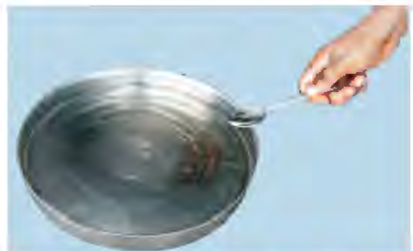
Fig. 5.4 : Vibrating Plate Produces Waves in Water
