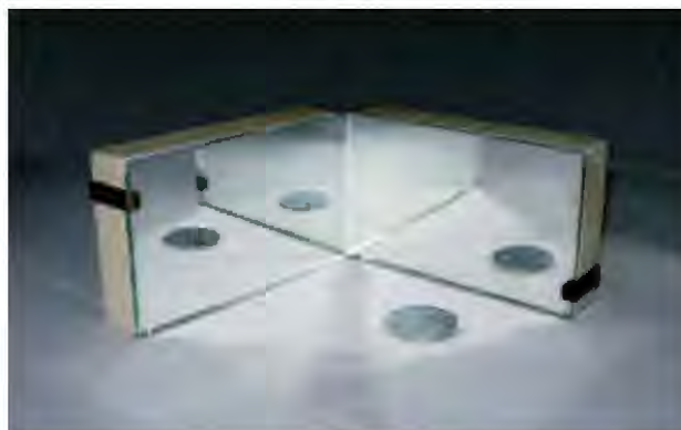
Fig. 12.10 : Images In Plane Mirror at Right Angle to Each Other
