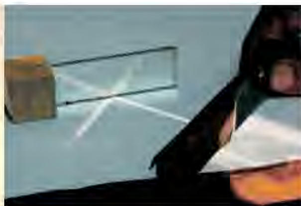
Fig. 12.1 : Arrangement for Showing Reflection
