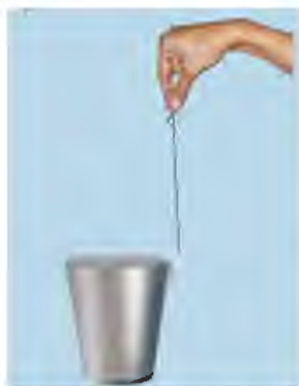
Fig. 5.17 : Thermocole Ball Touching the Vibrating Glass Tumbler
