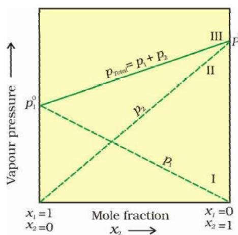
**Fig. 2.3:** The plot of vapour pressure and mole fraction of an ideal solution at constant temperature. The dashed lines I and II represent the partial pressure of the components. (It can be seen from the plot that  $p_1$  and  $p_2$  are directly proportional to  $x_1$  and  $x_2$ , respectively). The total vapour pressure is given by line marked III in the figure.
