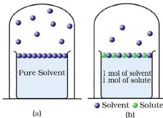
**Fig. 2.4:** Decrease in the vapour pressure of the solvent on account of the presence of solute in the solvent (a) evaporation of the molecules of the solvent from its surface is denoted by ●, (b) in a solution, solute particles have been denoted by ● and they also occupy part of the surface area.
