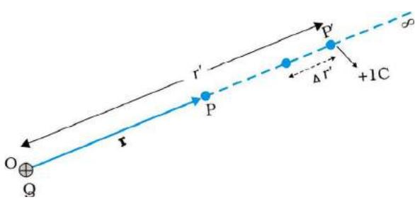
**FIGURE 2.3** Work done in bringing a unit positive test charge from infinity to the point  $P$ , against the repulsive force of charge  $Q$  ( $Q > 0$ ), is the potential at  $P$  due to the charge  $Q$ .
