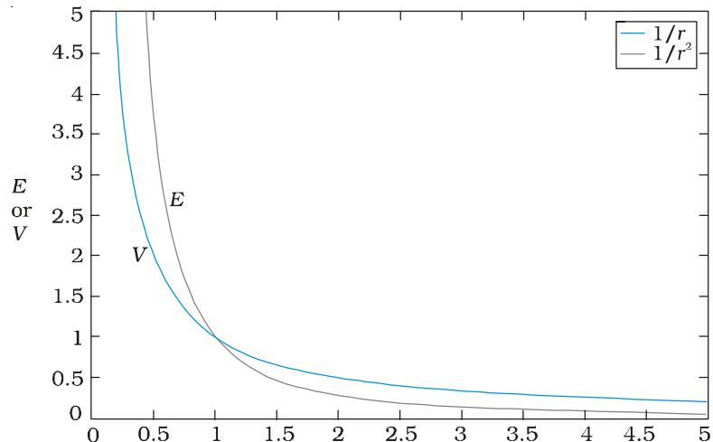
**FIGURE 2.4** Variation of potential  $V$  with  $r$  [in units of  $(Q/4\pi\epsilon_0) \text{ m}^{-1}$ ] (blue curve) and field with  $r$  [in units of  $(Q/4\pi\epsilon_0) \text{ m}^{-2}$ ] (black curve) for a point charge  $Q$ .
