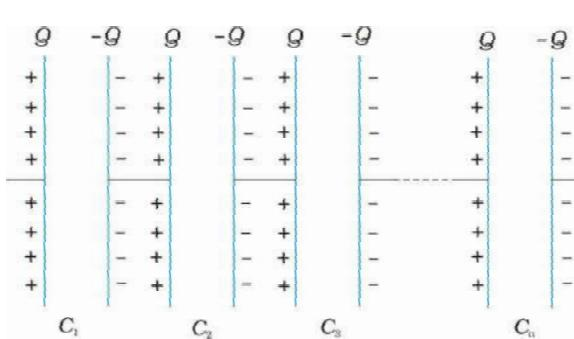
**FIGURE 2.27** Combination of  $n$  capacitors in series.
