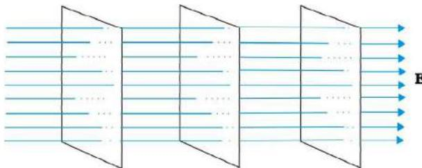
**FIGURE 2.10** Equipotential surfaces for a uniform electric field.
