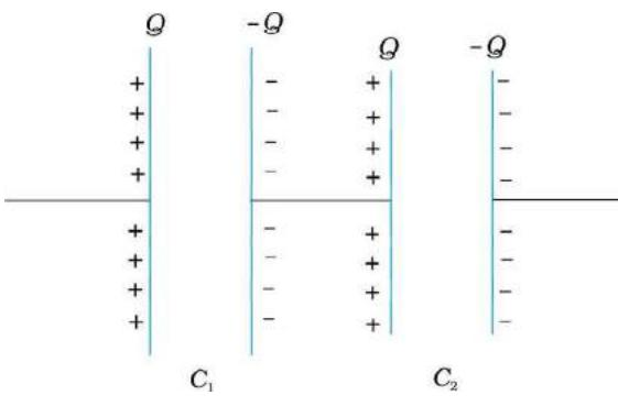
**FIGURE 2.26** Combination of two capacitors in series.
