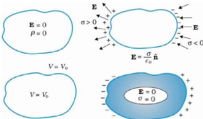
**FIGURE 2.19** Some important electrostatic properties of a conductor.
