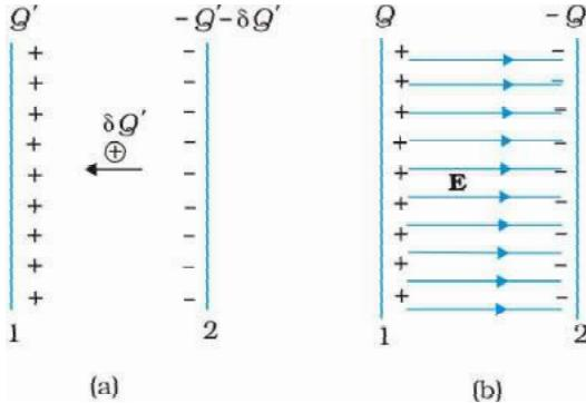
**FIGURE 2.30** (a) Work done in a small step of building charge on conductor 1 from  $Q'$  to  $Q'+\delta Q'$ . (b) Total work done in charging the capacitor may be viewed as stored in the energy of electric field between the plates.
