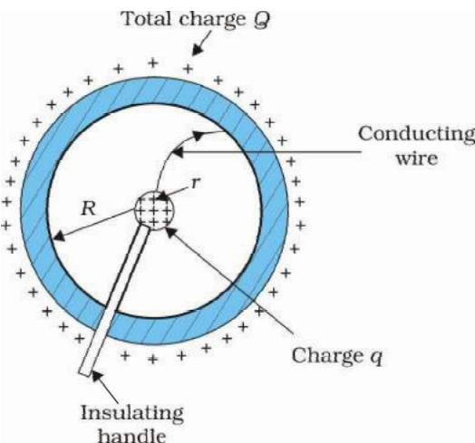
**FIGURE 2.32** Illustrating the principle of the electrostatic generator.
