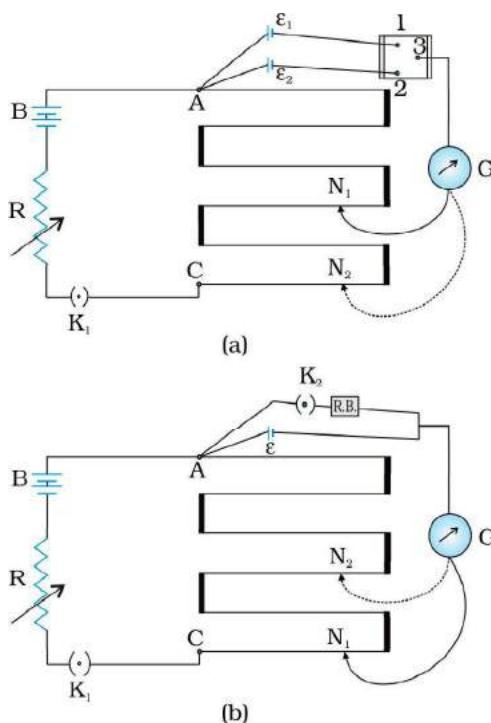
**FIGURE 3.28** A potentiometer.  $G$  is a galvanometer and  $R$  a variable resistance (rheostat). 1, 2, 3 are terminals of a two way key
