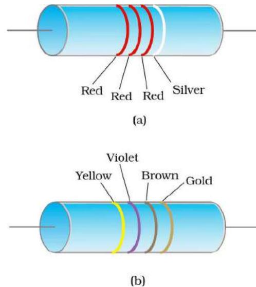
**FIGURE 3.8** Colour coded resistors
