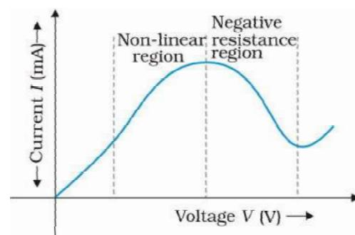
**FIGURE 3.7** Variation of current versus voltage for GaAs.
