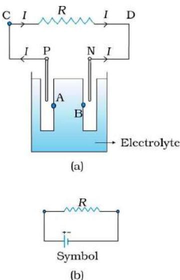
**FIGURE 3.18** (a) Sketch of an electrolyte cell with positive terminal P and negative terminal N. The gap between the electrodes is exaggerated for clarity. A and B are points in the electrolyte typically close to P and N. (b) the symbol for a cell, + referring to P and - referring to the N electrode. Electrical connections to the cell are made at P and N.
