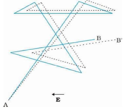
**FIGURE 3.3** A schematic picture of an electron moving from a point A to another point B through repeated collisions, and straight line travel between collisions (full lines). If an electric field is applied as shown, the electron ends up at point B' (dotted lines). A slight drift in a direction opposite the electric field is visible.
