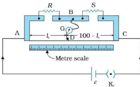
**FIGURE 3.27** A meter bridge. Wire AC is 1 m long.  $R$  is a resistance to be measured and  $S$  is a standard resistance.
