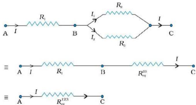
**FIGURE 3.17** A combination of three resistors  $R_1$ ,  $R_2$  and  $R_3$ .  $R_2$ ,  $R_3$  are in parallel with an equivalent resistance  $R_{eq}^{23}$ .  $R_1$  and  $R_{eq}^{23}$  are in series with an equivalent resistance  $R_{eq}^{123}$ .
