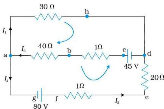
**FIGURE 3.22** At junction a the current leaving is  $I_1 + I_2$  and current entering is  $I_3$ . The junction rule says  $I_3 = I_1 + I_2$ . At point h current entering is  $I_1$ . There is only one current leaving h and by junction rule that will also be  $I_1$ . For the loops 'ahdeba' and 'ahdefga', the loop rules give  $-30I_1 - 41I_3 + 45 = 0$  and  $-30I_1 + 21I_2 - 80 = 0$ .
