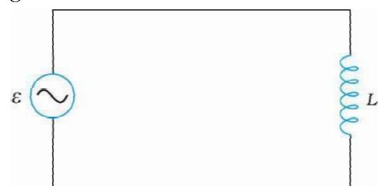
**FIGURE 7.5** An ac source connected to an inductor.
