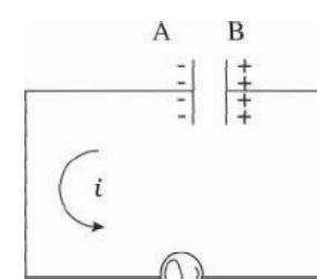
**2-3** As  $i$  continues to flow from A to B, the capacitor is charged to reversed polarity i.e., the plate B acquires positive and A acquires negative charge. Both the current and the voltage are negative. Their product  $p$  is positive. The capacitor ABSORBS ENERGY during this 1/4 cycle.
