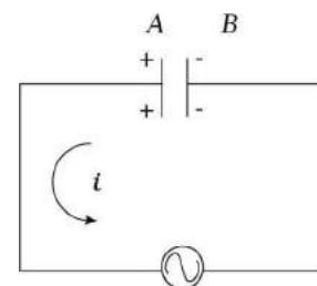
**0-1** The current  $i$  flows as shown and from the maximum at 0, reaches a zero value at 1. The plate A is charged to positive polarity while negative charge  $q$  builds up in B reaching a maximum at 1 until the current becomes zero. The voltage  $v_c = q/C$  is in phase with  $q$  and reaches maximum value at 1. Current and voltage are both positive. So  $p = v_c i$  is positive. ENERGY IS ABSORBED FROM THE SOURCE DURING THIS QUARTER CYCLE AS THE CAPACITOR IS CHARGED.
