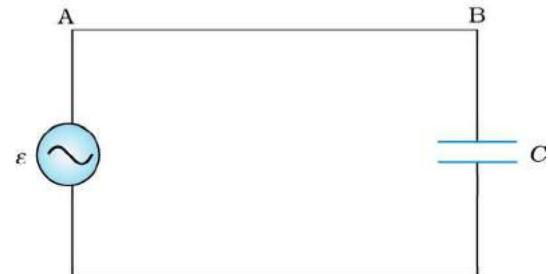
**FIGURE 7.8** An ac source connected to a capacitor.
