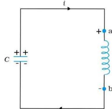
**FIGURE 7.18** At the instant shown, the current is increasing so the polarity of induced emf in the inductor is as shown.
