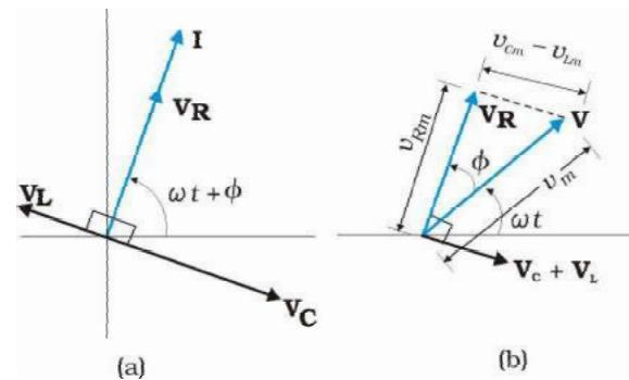
**FIGURE 7.13** (a) Relation between the phasors  $\mathbf{V}_L$ ,  $\mathbf{V}_R$ ,  $\mathbf{V}_C$ , and  $\mathbf{I}$ . (b) Relation between the phasors  $\mathbf{V}_L$ ,  $\mathbf{V}_R$ , and  $(\mathbf{V}_L + \mathbf{V}_C)$  for the circuit in Fig. 7.11.
