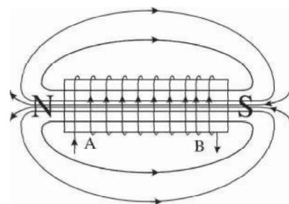
**0-1** Current  $i$  through the coil entering at A increase from zero to a maximum value. Flux lines are set up i.e., the core gets magnetised. With the polarity shown voltage and current are both positive. So their product  $p$  is positive. ENERGY IS ABSORBED FROM THE SOURCE.
