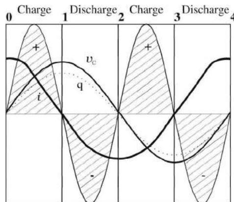
One complete cycle of voltage/current. Note that the current leads the voltage.
