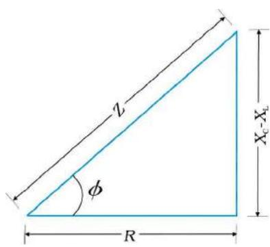
**FIGURE 7.14** Impedance diagram.
