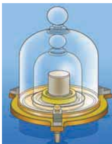
Figure 1.7 The international 1 kg standard of mass, a platinum-iridium (9:1) cylinder 3.9 cm in height and diameter.
