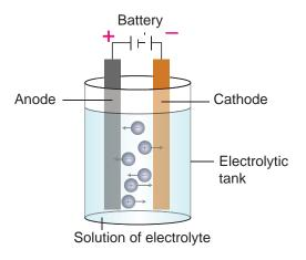
Figure 5.16 Electrolytic Cell
