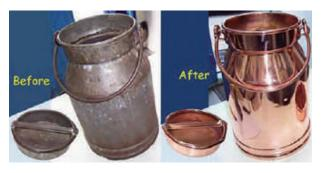
Figure 5.17 Chromium plating on iron
