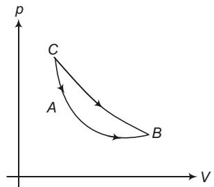
$$\begin{aligned} p_0^2 V_0 &= \frac{p_0}{2} V^2 = V \cdot 4V_0 \\ T &= \frac{\frac{p_0}{2} 4V_0}{nR} = 2 \frac{p_0 V_0}{nR} = 2T_0 \\ U &= nC_V T = 2 \cdot \frac{3}{2} R (2T_0 - T_0) \\ &= 3R \frac{p_0 V_0}{2R} = \frac{3}{2} p_0 V_0 \end{aligned}$$
