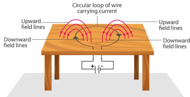
For the downward direction of the current, the direction of the magnetic field will be as if emerging from the table outside the loop and merging to the table inside the loop. Similarly, for current flowing in the upward direction, the direction of the magnetic field will be as if they are emerging from the table outside the loop and merging to the table inside the loop as shown in the figure.
