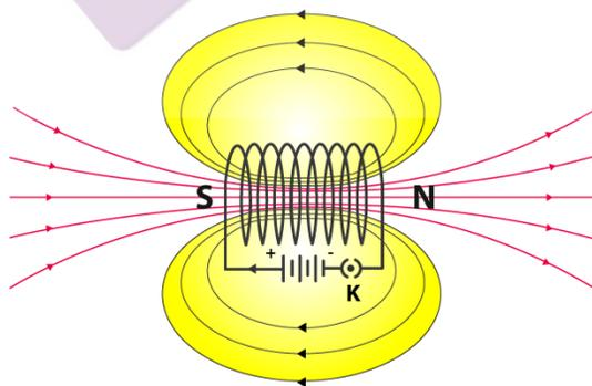
When the north pole of the bar magnet is brought close to the end connected to the negative terminal of the battery, the solenoid repels the battery. As like poles repel each other, we can infer that the end connected to the negative terminal behaves as a north pole while the end connected to the positive terminal behaves as a south pole.
