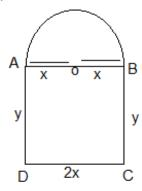
Perimeter of window = Semi-circular arc AB + Length (AD + DC + BC)
