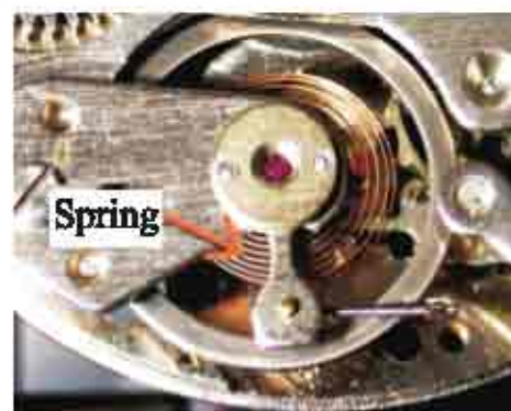
(b) Internal view of spring loaded watch.
