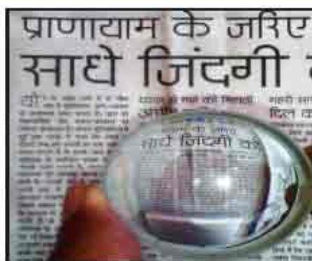
Fig. 14. 10 small, erect and virtual image formation by concave lens.
