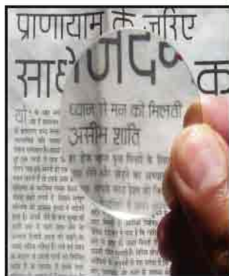
Fig. 14.9(b) Big, erect and virtual image formation through convex lens.
