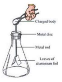
It consists of a metal rod on which two leaves of aluminium foil are fixed to one end and a metal disc at the other end. The leaves are kept inside a conical flask and it is corked to isolate it from the atmospheric air.
