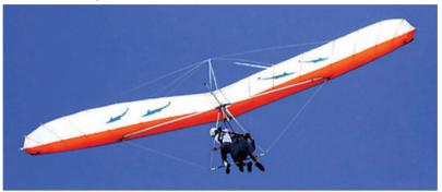
Most modern hang-gliders are made of aluminium alloy. The pilot is safe when fastened to a harness suspended from the frame of the glider.
