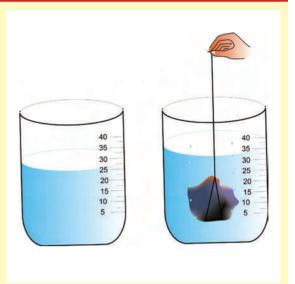
Let us find the volume of a stone using a measuring cylinder.
