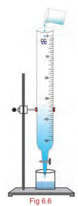
Used to make a small fixed volume of liquid to flow.
