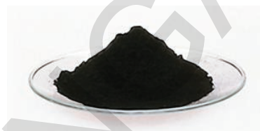
fig-15(a): Copper Oxide change into black colour
