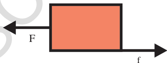
Fig-11: Horizontal forces on the brick
