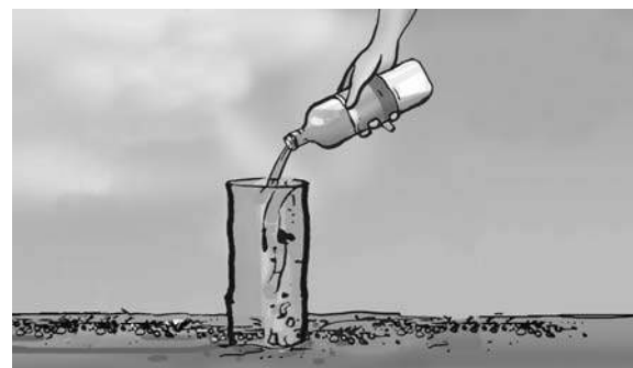
Fig. 9.5 Measuring rate of percolation
