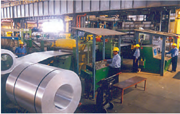
Fig. 6.6: Strip casting mill at smelter of NALCO
