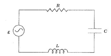
Figure shows a ideal series LCR circuit connected to a.c. mains of voltage  $\epsilon$ ,
