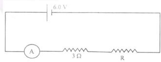
When the circuit is switched on, the ammeter reads 0.5 A.
