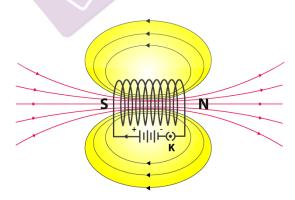
When the north pole of the bar magnet is brought close to the end connected to the negative terminal of the battery, the solenoid repels the battery. As like poles repel each other, we can infer that the end connected to the negative terminal behaves as a north pole while the end connected to the positive terminal behaves as a south pole.
