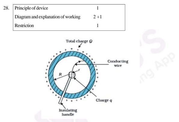
Principle: The inner smaller sphere is at a higher potential than the larger outer sphere. Hence even a small positive charge, on the small sphere, flows immediately to the larger sphere when both are connected by a conducting wire, even when the charge on the larger sphere is quite large.
