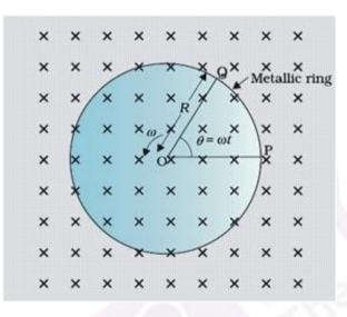
The magnitude of the emf, generated across a length dr of the rod, as it moves at right angles to the magnetic field, is given by
