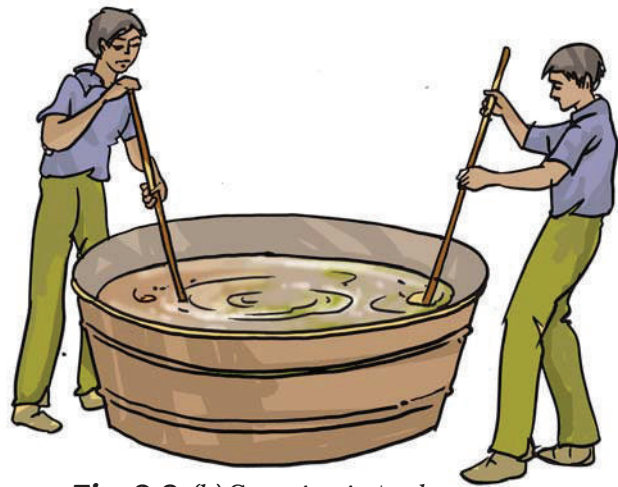
Fig. 3.8 (b) Scouring in tanks
