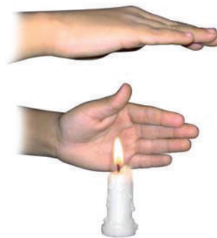
Fig. 4.10 Transfer of heat by convection in air
