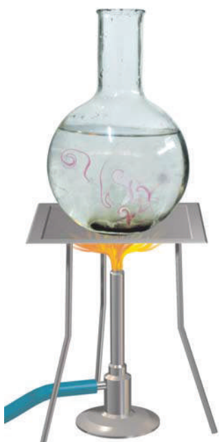
Fig. 4.9 Convection of heat in water
