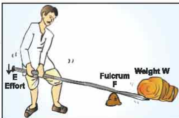
Figure 11.3 (a): Lifting weight with a crowbar
