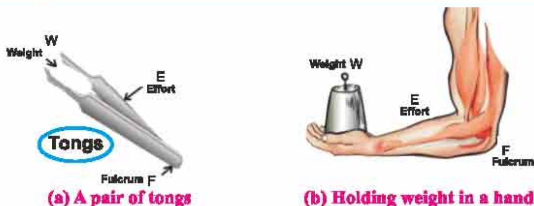
Figure 11.8 Examples of third order levers
