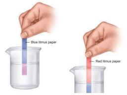
Figure 14.3 Test for acid and base using litmus paper
