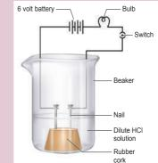
of a 6V battery through a bulb and a switch as shown in Figure. Now pour some dilute HCl in the beaker and switch on the current. Repeat the activity with dilute sulphuric acid, glucose and alcohol solutions.What do you observe now? Does the bulb glow in all cases?
