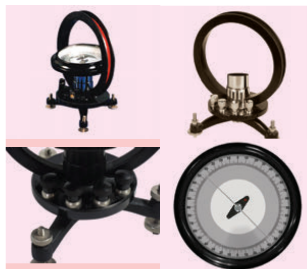
Figure 3.22 Tangent Galvanometer and its parts
