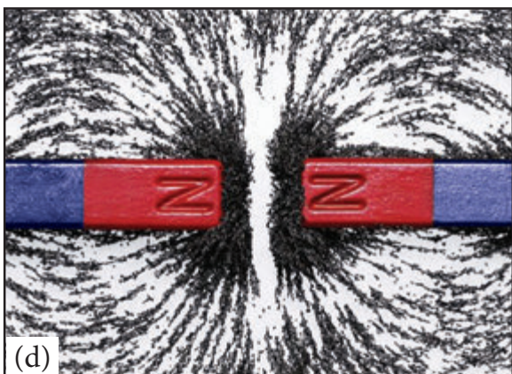
Figure 3.10 Properties of magnetic field lines– unlike poles attracts each other shown in picture (a) and (b) like poles repel each other–shown in picture (c) and (d)
