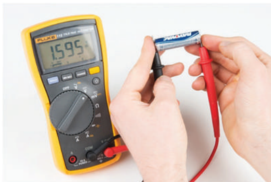
Figure 2.19 Measuring the emf of a cell
