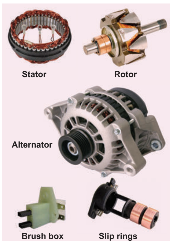
Figure 4.27 AC generator and its components
