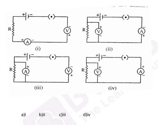
36 The current through the resister connected in an electric circuit and the potential 1 difference across its ends are shown in the diagram.
