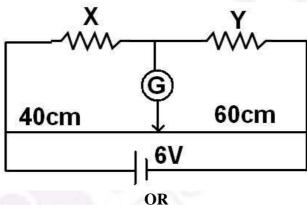
Calculate the current drawn from the battery in the given network shown here. State Kirchhoff's loop law and name the law on which it is based on.
