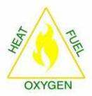
The diagram given represents what is called the **fire triangle** which shows that oxygen, heat and fuel in the proper proportions are necessary to create a fire. Reducing or eliminating any or all of these properly can help in containing or stopping the fire.
