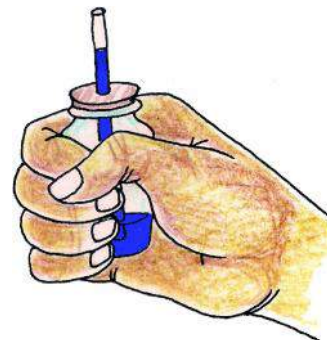
Figure-2: Homemade thermoscope
