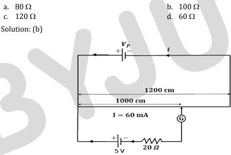
Assume the terminal voltage of the primary battery as  $V_p$ . As long as this potentiometer is operating on balanced length,  $V_p$  will remain constant.
