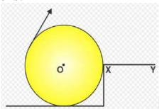
Force F should be applied in the direction as shown in the above figure.
