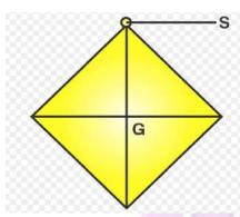
A square card board in rest position as centre of gravity as G and point of suspension as S
