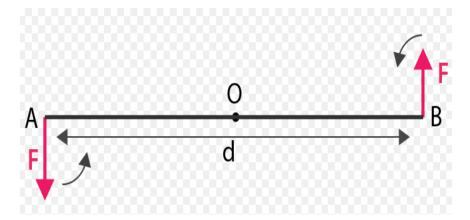
At A and B two forces each of magnitude F are applied, which are equal and opposite forces. The two forces rotate the bar in anticlockwise direction. AB is the perpendicular distance between two forces which is called the couple arm.
