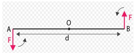
At A and B, two forces each of magnitude F are applied, which are equal and opposite forces. By observing the above figure it is clear that the two forces rotate the bar in anticlockwise direction.
