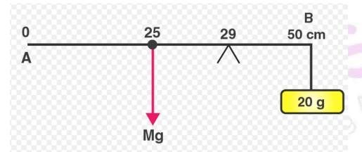
Figure shows a uniform half metre rule PQ which is balanced at 29 cm mark. Let the mass of the rule be M. A uniform rule has same distribution of mass throughout its length, so its weight Mg will act at its middle point which is at 25 cm. The weight mg produces anticlockwise moment about point O. To balance the 20g (0.02 kg) weight is tied at 50 cm mark which generates clockwise moment
