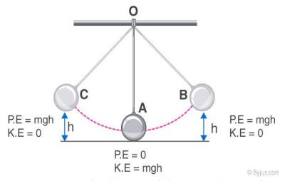
From B to A, again the potential energy changes into kinetic energy and this process repeat again and again. So, while swinging, the bob has the potential energy at the extreme position B or C and kinetic energy at resting position A. The bob has both the kinetic energy and potential energy at an intermediate position (between A and B or between A and C) and the sum of both the energies (i.e the total mechanical energy) remains constant throughout the swing.
