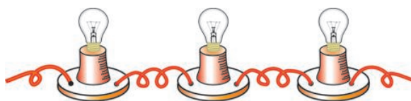
Fig. 12 - Bulbs connected in series
