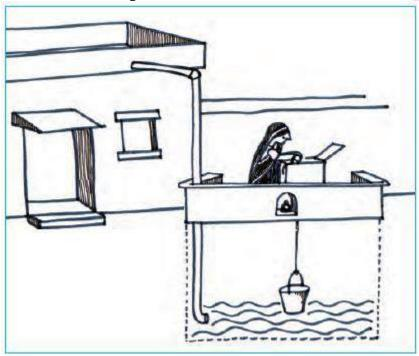
**Answer:** The water collected on the roof comes down in the pipes and gets stored in the tank below.
