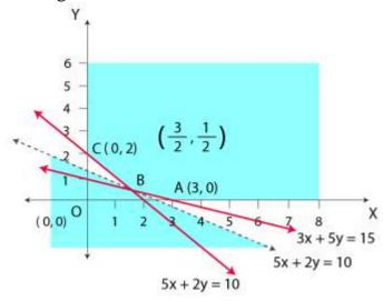
It can be seen that the feasible region is unbounded. The corner points of the feasible region are A (3, 0), B (3/2, 1/2) and C (0, 2) The values of Z at these corner points are given below
